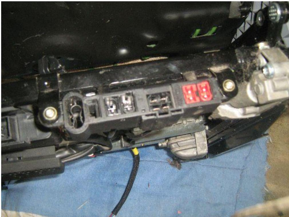
Then trace those wires back to the main module pop the back open and unplug the wires where they go into the control module
