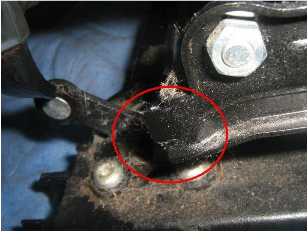
Then flip the seat over and remove the other side and the bolt into the seat belt latch. The plastic cover is held in by a small stud that locates into a hole. Just pull the back of the plastic towards the rear of the car and the stud pops out then you push it forward to detach the slot off the tang on the frame and wiggle it off the seat belt latch holder
