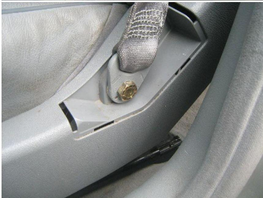
The seat in the right position pull out the rear covers on the seat rails – just finger pressure – to expose the bolts. The fronts are open. It takes a 12mm internal star
