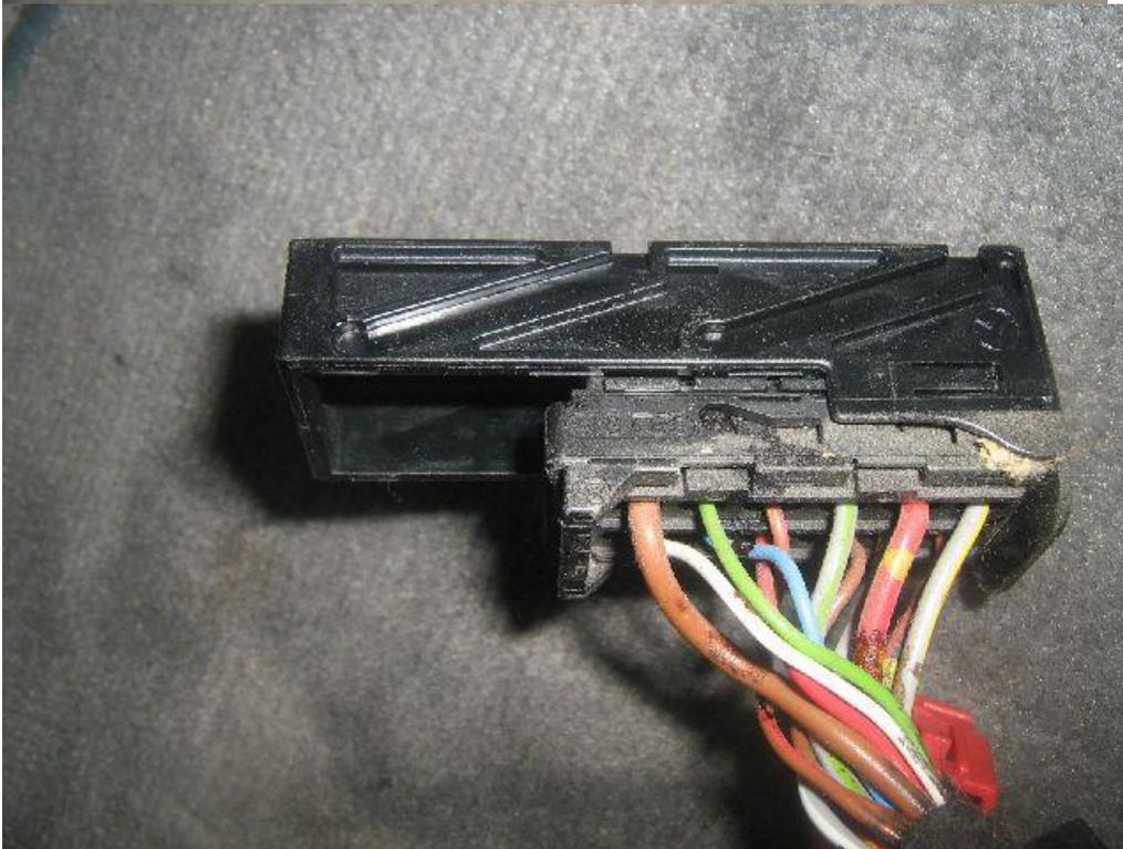
Then just lift out the seat. Make sure you have some blankets or similar on the floor to lay it on, you can also get at nthe wire connectors easier. Undo the 2 bolts and remove the small connector that has the seat heater wires in it.
